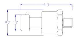
This pressure transmitter is to be powered by regulated 5 VDC power supply. Connect red wire to the 5VDC power source. Connect black wire to the ground. Blue wire is the signal output.
